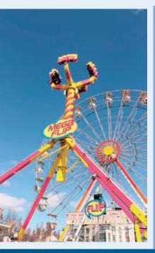
With high marketability, lots of fun and suitable for large public it is our entry level thrill pendulum ride. This ride has two exciting elements: ±360° arch with boosted fall and gondolas spin at variable speeds. Large and comfortable seats with a big back shield for themeng purpose, silent and maintence free transmission without pinion and high tech control system with double drive make this ride a top class choice in comparision with any competitor.
